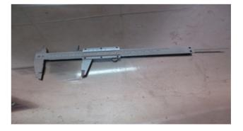
Figure 2 Vernier caliper gauge.
