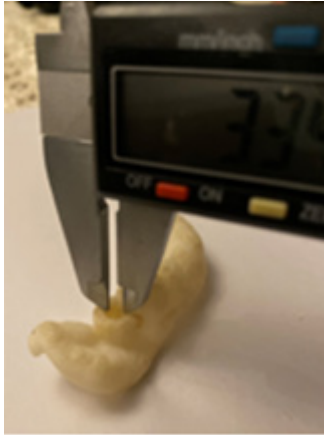
Figure.4 showing measuring guide tube diameter using digital caliber
